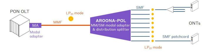
As far as the SM to MM version is concerned, the principle remains the same. Downstream, AROONA-POL splits the SMF signal from OLT and converts it to the LP $_{\rm 01}$  distribution
