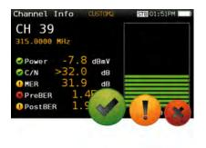
Reduce installation mistakes with the on-screen Pass/Fail indicators, a graphical tool that helps and speeds up the interpretation of measurement results. Different thresholds are available depending on the network area to be analysed: headend, multi-band amplifiers, bridging connection, connection records, user home, etc. Besides the pre-set values, you will be able to customize your own threshold values.
