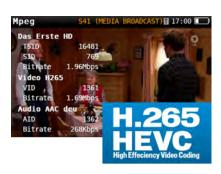
This functionality supports HEVC H.265 new compression format and allows to display video signals with a maximum Full HD resolution (1920 x 1080). Information can be displayed both on the meter screen\* or on the mobile device (multiscreen mode) as long as your hardware is H.265 compatible (usually a smartphone, tablet or PC). (\*) Optional function: Ref. 593252
