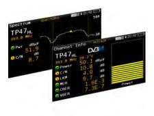
This functionality for DVB-S/S2 allows the complete analysis of a satellite channel in any frequency within the 250 MHz to 2300 MHz range. Thus, the meter can be directly connected to any output of a LNB Wideband (2 outputs: Vertical and Horizontal)
