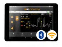
Equipped with 2.4/5 GHz Wi-Fi and Bluetooth, the equipment allows a secure access through an Android or iOS device, or a PC. In this way, the WEB management application may be used to query and edit channel plans or user profiles, export measurements, etc.
