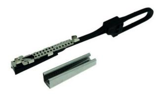
Part of the Telenco® HYPOCLAMP family, the HYPOCUT clamp enables the anchoring of flat aerial drop cables where spans do not exceed 70m. This clamp consists of a stainless steel body, a shim with an embedded blade and a plastic wedge equipped with an integrated opening bail. For easy cable installation, the Telenco® HYPOCUT clamp is delivered in 2 parts.
