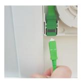
12. Using the 1m Connection Patch Lead, connect the internal Squebble to the active kit.
