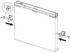
Note: Whenever possible, attach two screws into wall studs. If stud mounting is not possible, use an expandable wall anchor. Hardware is not included; .25" x 2" lag bolts are recommended. Mount the UPS in either of the displayed positions.
