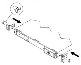
**S** Secure clip-nuts to the rack, and attach brackets with provided screws.
