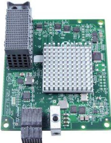
Figure 1. IBM Flex System FC3172 2-port 8Gb FC Adapter
