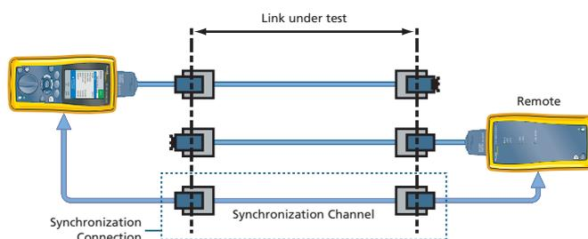
Figure 3. Pair-to-pair Alien FEXT measurements. The main and remote units are plugged into different cabling links at opposite ends of the bundle under test. A spare channel in this bundle connects the synchronization modules plugged into each of the testers to allow the testers to perform all of the pair-to-pair FEXT measurements between the wire pairs of two selected cabling links.
